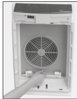
2. Grasp the UV lamp and rotate it by 90°. Now it can be pulled out.
