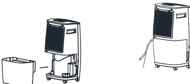
3.4. Proper drainage of the condensation water with hose connection ! Make sure that the hose always has a slight downward slope (see following diagrams).
